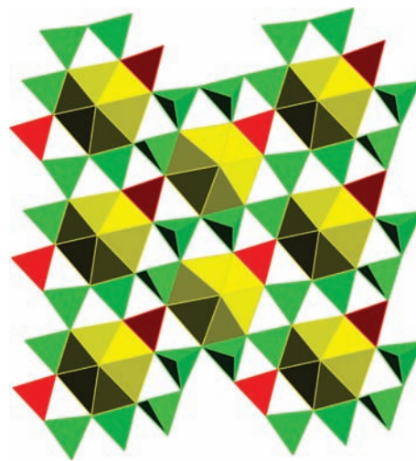
Figure 2. View along the b axis of the actinyl borate sheets in \text{AnO}_2[\text{B}_8\text{O}_{11}(\text{OH})_4] (An = U, Np, Pu). \text{AnO}_8 hexagonal bipyramids are shown in yellow, \text{BO}_3 triangles in red, and \text{BO}_4 tetrahedra in green.
